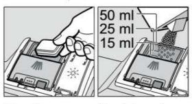
Close the cover on the detergent dispenser by sliding it up until the lock engages without difficulty.
